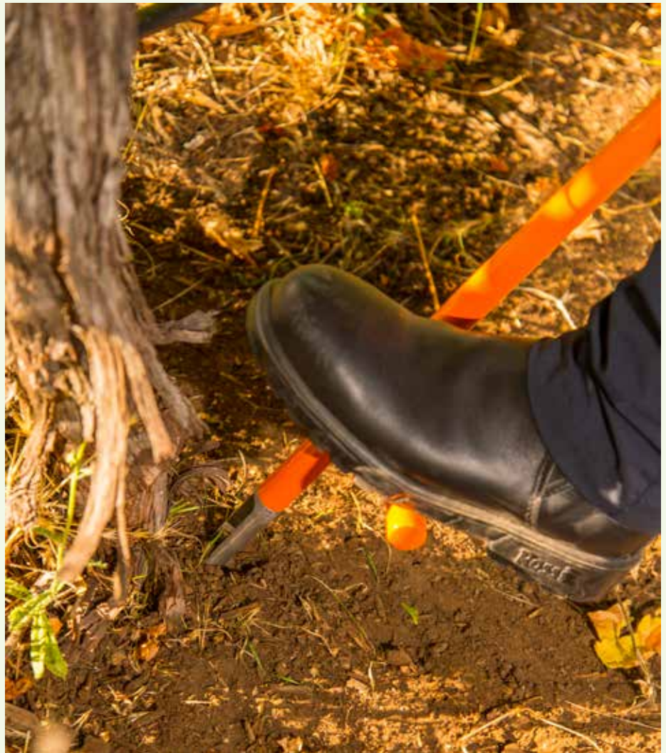
Collecting a soil sample for the DNA method using a soil corer. Image courtesy Vinehealth Australia
