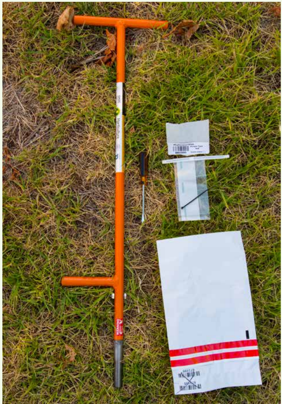
Components of the soil sampling kit for collecting soil cores for the DNA method. Image courtesy Vinehealth Australia
