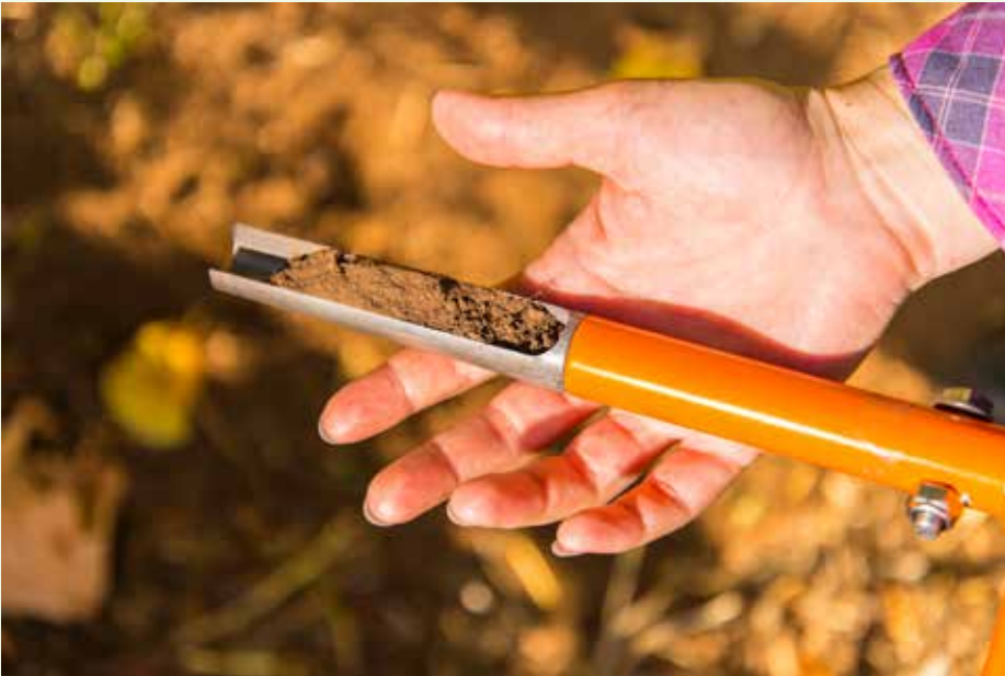
A soil core collected as part of the DNA phylloxera detection method. Image courtesy Vinehealth Australia
