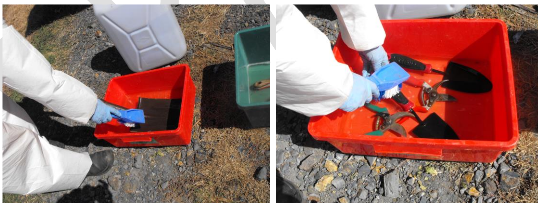
Figure 10. Use a brush to remove soil from shovels, trowels and secateurs in 2% sodium hypochlorite .
