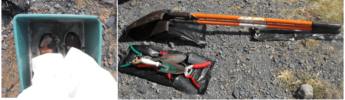
Figure 11. Dip footwear, shovels, trowels and secateurs in 2% sodium hypochlorite solution and dry on a black surface.
