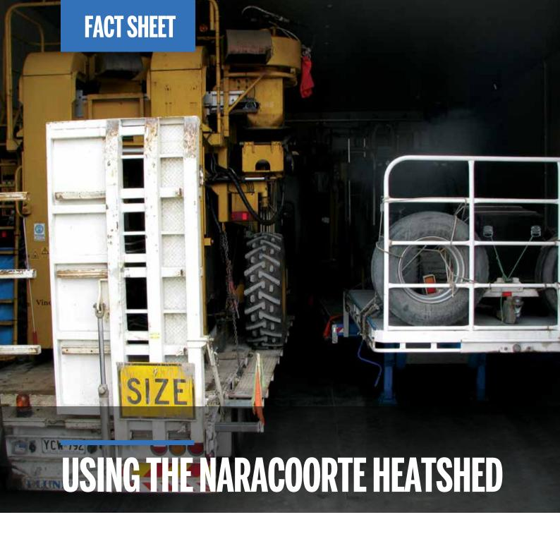
Machinery and equipment are high risk vectors for spreading weeds, diseases and pests such as phylloxera, as they can carry grapevine material and soil and are especially hard to clean. The only way to ensure machinery and equipment is free of pests, diseases and weeds is to 'bake it' in a heat shed.
